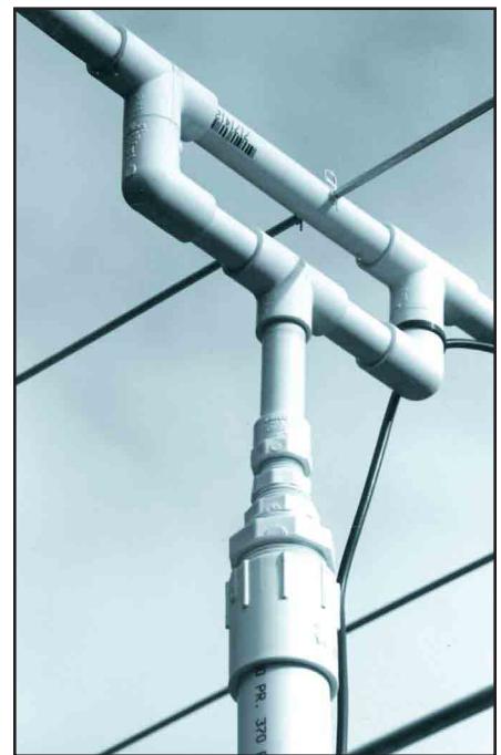
Figure 6—A close-up view of the parallel PVC boom and mount, the sequence of threaded fittings and the hitch-pin clips used to secure the parasitic elements.
